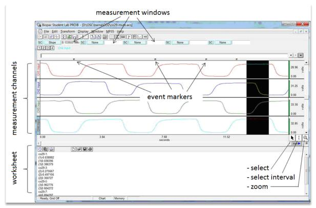
2. Defining the input channels (MP36/Set up channels ...)
